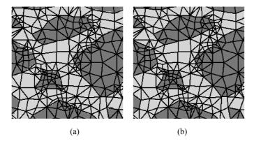
Figure 4 A detail (a) of the *Skeleton* from Figure 3, with additional refinement and (b) the same detail, with elements coloured according to their dominant *Material*
