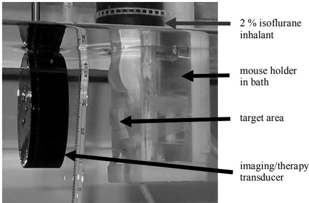
Figure 1. Pulsed HIFU treatment of mouse flank in a water bath.
