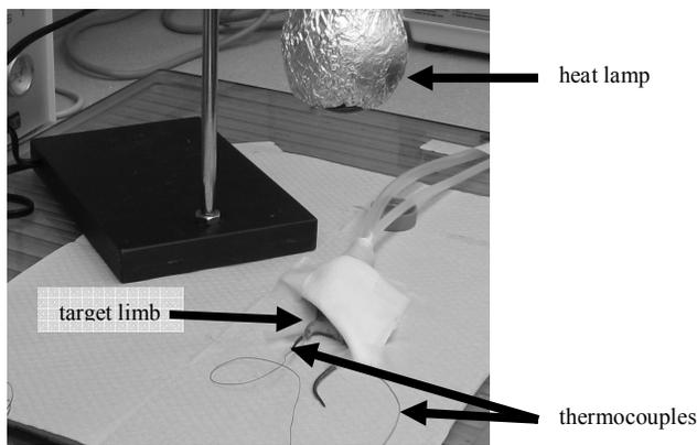
Figure 3. HT treatment setup. Heating in the limb is monitored with interstitial hypodermic thermocouples and manually adjusted by controlling the current through the heat lamp.
