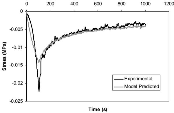
**Figure 1. The model vs. experimental stress for the second load cycle of sample 5.**
