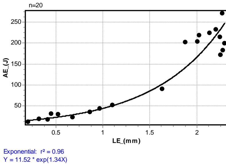
Figure 10. AE versus LE data for the two treatments of cast steel.
