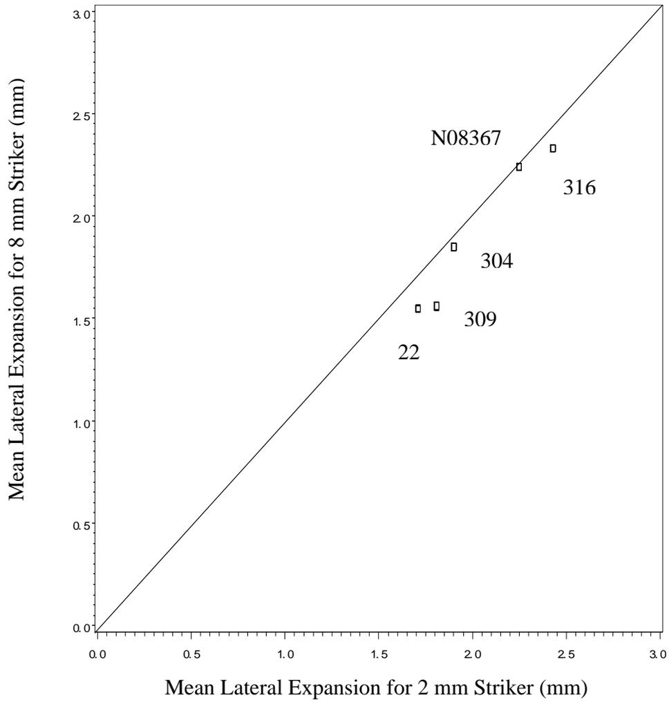
Figure 5. Lateral expansion means when tested by the two striker designs. Each point represents data from a single alloy when tested by the strikers.
