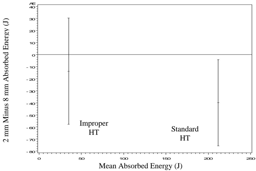
Figure 4. Graphical representation of the differences in the means for the data in Table 2.
