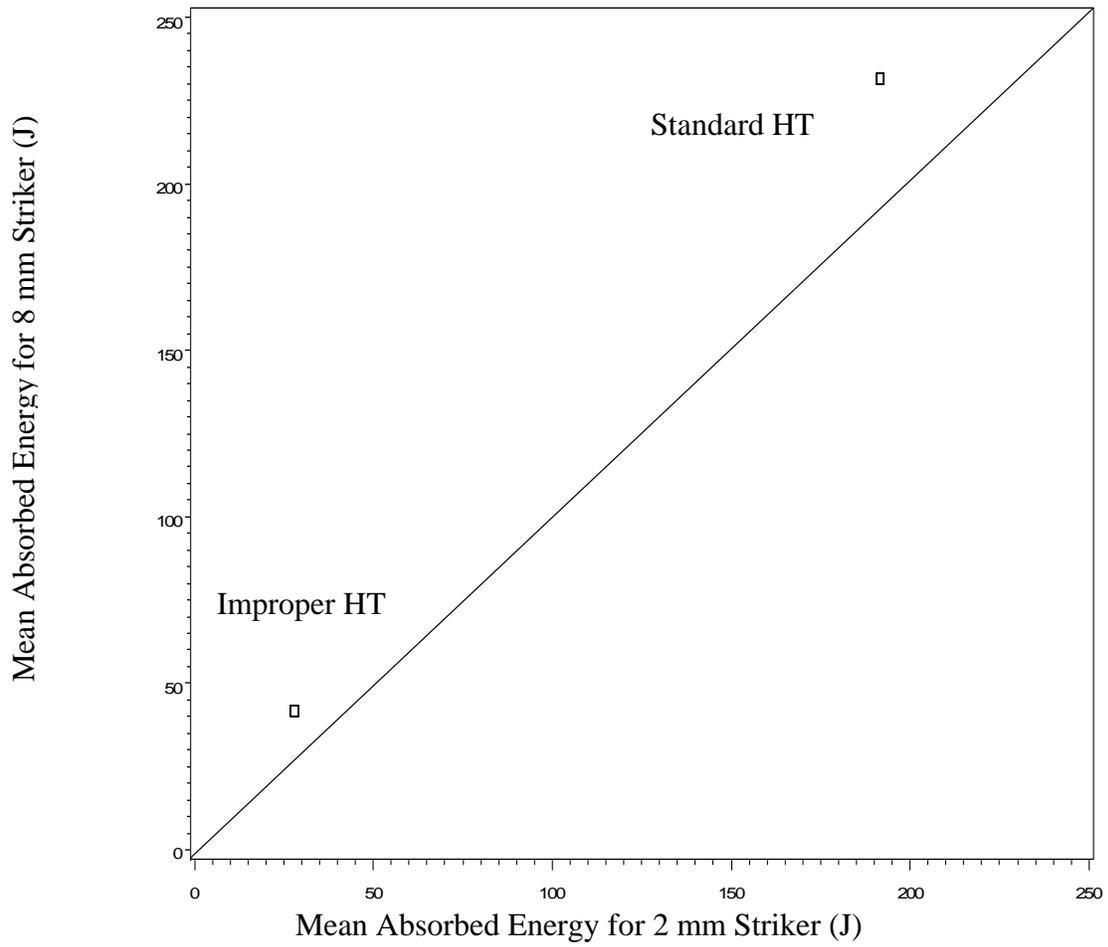
Figure 3. Absorbed energy means for cast alloys when tested by the two striker designs. Each point represents data from a single heat treatment condition when tested by each striker.
