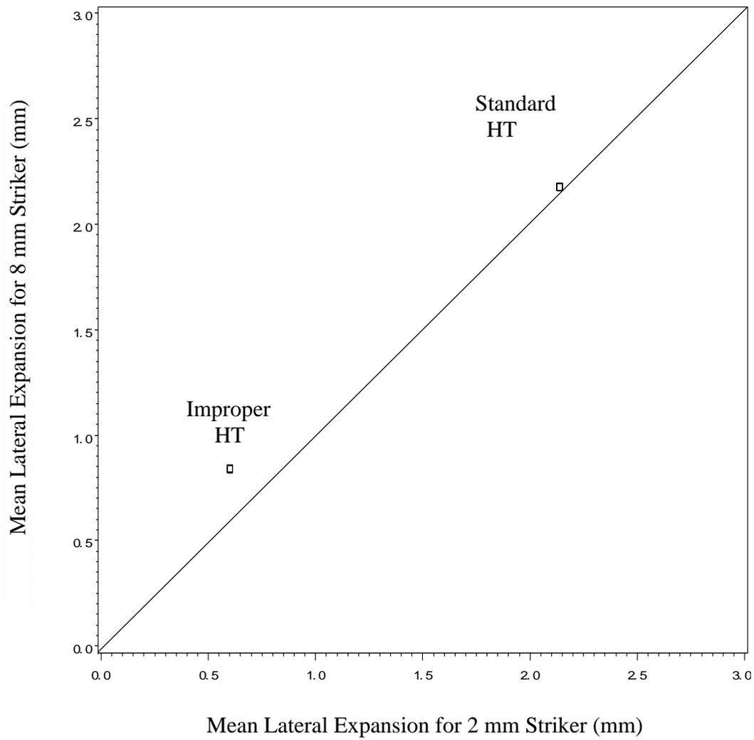
Figure 7. Lateral expansion means for cast alloys when tested by the two striker designs. Each point represents data from a single heat treatment condition when tested by each striker.
