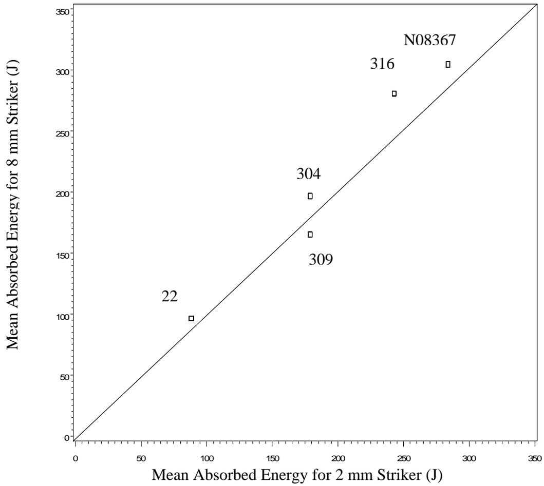
Figure 1. Absorbed energy means when tested by the two striker designs. Each point represents the sample mean for a single alloy when tested by the 8 and 2 mm strikers.
