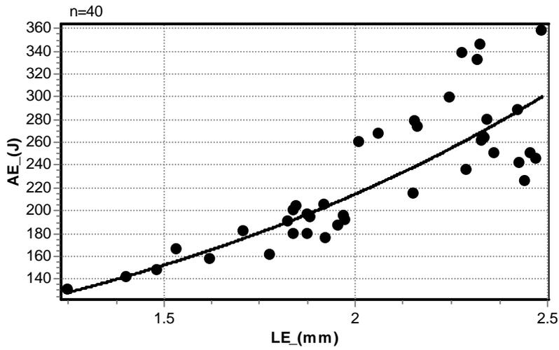
Figure 9. AE versus LE data for four wrought stainless steels (304, 309, 316, and N08367).
