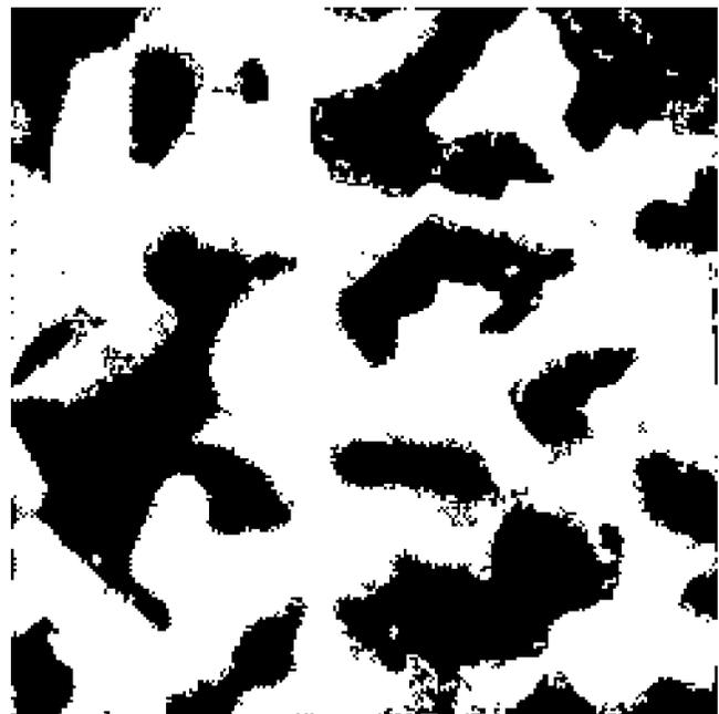
**Figure 3.** The material map (a 1 mm  $\times$  1 mm slice) for the finite element model of the porous PCL scaffold. Black indicates a pore.
