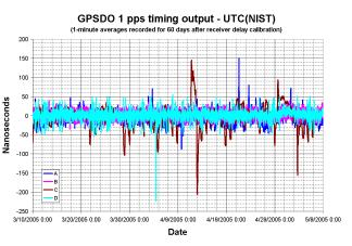
Figure 2. Phase plot of GPSDO 1 pps – UTC(NIST) using known antenna coordinates.
