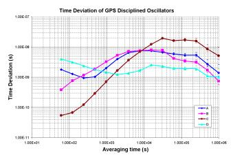
Figure 4. Time stability of GPSDO 1 pps outputs.
