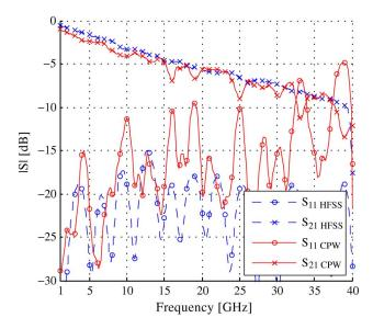
Fig. 3. Simulated scattering (S) parameter performance of optimized CPW flex to chip launch, in blue dashed lines, compared to measured cryoprobe with CPW flex through line results from Section III, in red solid lines.
