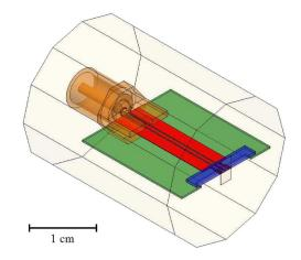
Fig. 2. Broadband flip-chip-on-flex interface model in HFSS. From left to right, yellow is the FEM domain boundary, orange is the Cu connector, white is PTFE, green is the RO3006, red is copper traces, yellow is InSn solder, blue is the Si chip, and maroon is Nb traces on-chip.
