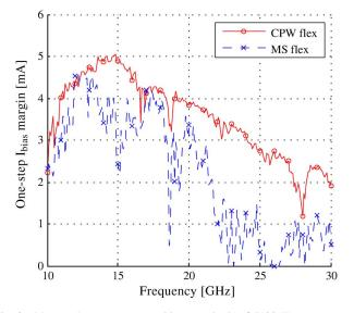
Fig. 8. Measured one-step current bias magnitude of 5120-JJ arrays on two identical ACJVS chips mounted in different "flip-chip on flex" packages. The improved CPW package data set is shown in red solid lines marked with  $\circ$ ; the legacy MS package data set is shown in blue dashed lines marked with  $\times$ . A larger one-step magnitude is an indication of better microwave power uniformity across all the junctions in the array.
