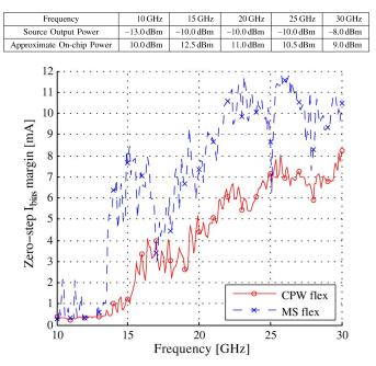
Fig. 7. Measured zero-step current bias magnitude of 5120-JJ arrays on two identical ACJVS chips mounted in different "flip-chip on flex" packages. The improved CPW package data set is shown in red solid lines marked with  $\circ$ ; the legacy MS package data set is shown in blue dashed lines marked with  $\times$ . Zero-step suppression below  $I_C$  of 11.5 mA is an indication of absolute microwave power reaching any one junction in the array.
