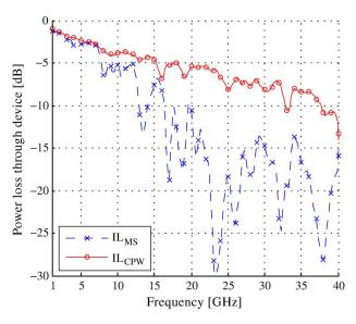
Fig. 5. Measured cryoprobe RL, using room-temperature SOLT calibration, of MS legacy flex package in blue dashed lines, and CPW-optimized flex package in red solid lines.
