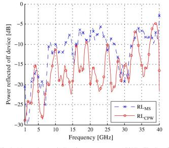
Fig. 4. Measured cryoprobe IL, using room-temperature SOLT calibration, of MS legacy flex package in blue dashed lines, and CPW optimized flex package in red solid lines.
