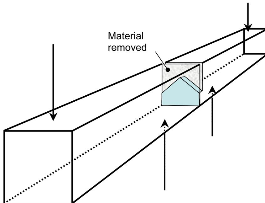
Figure 1. Conventional chevron-notch test structure. The forces are applied at the four points shown.
