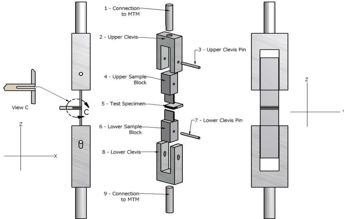
Figure 3. Suggested configuration for interfacing the micro-chevron to a materials testing machine.
