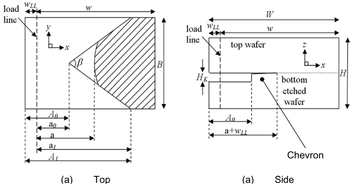
Figure 2. Key dimensions of the micro-chevron test structure described in MS5-1107. The recommended values of  $W$  and  $B$  are 10 mm each.
