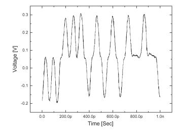
Fig. 1. Typical pulse shapes from the pattern generator showing different pulse shapes and amplitudes depending on their location in the pulse pattern.
