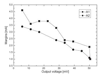
Fig. 3. Operating margins as a function of the output voltage for two different broadband amplifiers (A1 and A2). The output voltage is chosen by setting the fraction of peak amplitude between 10 % and 90 % by means of the delta–sigma algorithm. Measurements were done with Chip II using one array.
