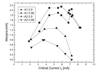
Fig. 2. Operating margins versus critical current of a single array from Chip I for two different output voltages and two different amplifiers. The amplifiers (A1 and A2) with different gain and bandwidth were used to amplify the ternary pulse signal. Waveforms with two different peak amplitudes (0.9 and 0.98) generated voltages at either 100 mV or 110 mV.
