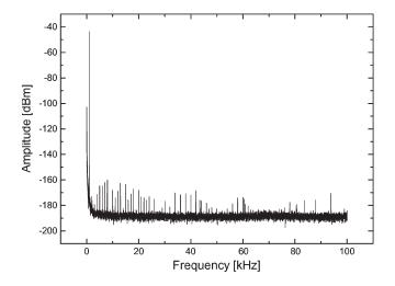
Fig. 5. Spectrum of a 200 mV, 1 kHz signal showing the intrinsic low distortion from the digitizer at -110 dBc (ten averages, 2 Hz resolution bandwidth, 1 M $\Omega$  input impedance, 2 V input range). The residual peaks are from the distortion created by the digitizer.
