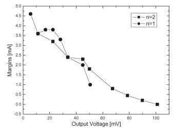
Fig. 4. Operating margins as a function of output voltage for the first (n = 1) and second (n = 2) Shapiro steps for the same range of fractions of peak voltage (10 % to 90 %). The output voltage is changed by means of the delta-sigma algorithm. Measurements were done with Chip II using one array. Amplifier A1 was used for these measurements.
