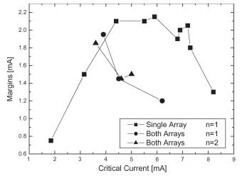
Fig. 6. Operating margins as a function of the critical current for the two array combined of Chip I as compared with the results for a single array (taken from Fig. 2). Measurements at n = 2 are done with 45 % fraction of the peak voltage.
