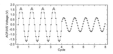
Fig. 7. Example of a dual juxtaposed ACPJVS waveform with n = 4 cycles of a 1.2 V rms and m = 4 cycles of 0.5-V rms sine waves, with a relative phase of 30°. For clarity, we show a waveform with only 16 samples per cycle.
