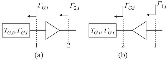
Fig. 1. (a) Forward and (b) reverse measurement configurations.
