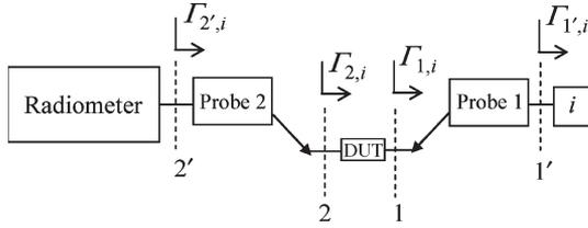
Fig. 2. Reference planes for on-wafer measurements.
