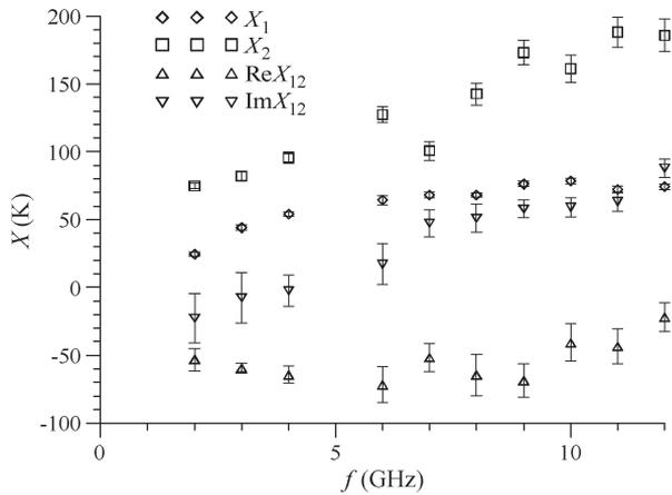
Fig. 3. Results and uncertainties for the  $X$ -parameters of a transistor on a wafer.
