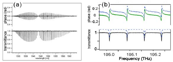
Figure 2(a) Measured phase and absorption spectrum for hydrogen cyanide (HCN). In total the measurement spanned from 1492 nm to 1618 nm or 155,000 individual frequency comb lines. For clarity only the data showing HCN absorption bands is shown. (b) Expanded view, data is in excellent agreement with previously published values [8] (dotted lines offset for clarity).
