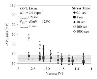
Figure 5:  $\Delta V_{TH}(ac)$  as a function of stress voltage for various stressing times. With the exception of the 1000 second stress, all of the stress induced  $\Delta V_{TH}$  is "recoverable".
