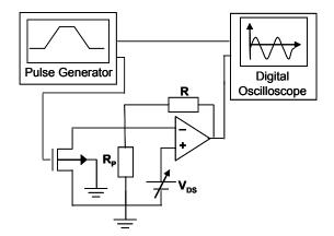
Figure 1. Fast- $I_{\rm D}V_{\rm G}$  experimental set-up using a pulse generator, digital oscilloscope, and fast amplifier circuit.
