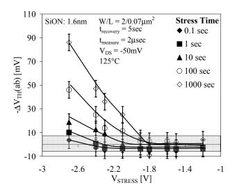
Figure 4:  $\Delta V_{TH}(ab)$  as a function of stress voltage for various stress times. It is clear that the fast NBTI degradation only occurs for exceedingly high stress voltages and longer stress times. The box centered about 0mV represents 1 standard deviation error bar. The lines are only a guide for the eye.
