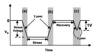
FIGURE 2: SCHEMATIC DIAGRAM OF THE GATE VOLTAGE PULSES DURING STRESS AND MEASUREMENT SEQUENCES.  $V_{TH}$  and  $G_M$  values are extracted at (A), (B), and (C).
