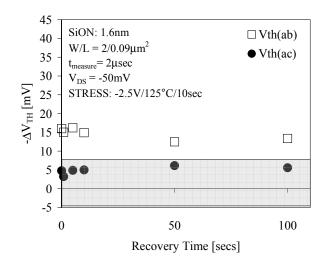
Figure 8:  $\Delta V_{TH}(ab)$  and  $\Delta V_{TH}(ac)$  as a function of recovery time. The box centered about 0 mV represents 1 standard deviation error bar.
