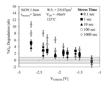
Figure 6: %G<sub>M</sub> degradation(ab) as a function of stress voltage for various stress times. The G<sub>M</sub> degradation(ab) follows a similar trend (large degradations only at high voltages) as  $\Delta V_{TH}(ab)$  (Figure 4). The box centered about 0 mV represents one standard deviation error bar.
