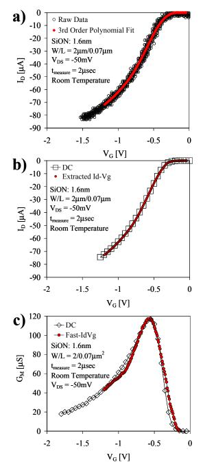
Figure 3: Our Fast- $I_DV_G$  characteristics are subject to significant noise. We utilize a "moving" third-order polynomial fitting procedure to extract the  $I_DV_G$  characteristic curves from the raw data (a). Our extracted  $I_DV_G$  (b) and  $G_M$  (c) characteristics agree very well with DC measurements.
