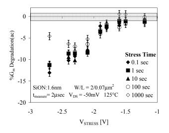
FIGURE 7: %GM DEGRADATION(ac) AS A FUNCTION OF STRESS VOLTAGE FOR VARIOUS STRESS TIMES. WE OBSERVE AN IMPROVEMENT IN  $G_M$  (BETTER THAN PRE-STRESS). THIS CAN BE EXPLAINED BY THE PRESENCE OF ELECTRON TRAPPING/DETRAPPING PHENOMENON. THE TRAPPED ELECTRONS CAN COMPENSATE POSITIVELY CHARGED INTERFACE TRAPS AND REDUCE THE COULOMBIC SCATTERING.
