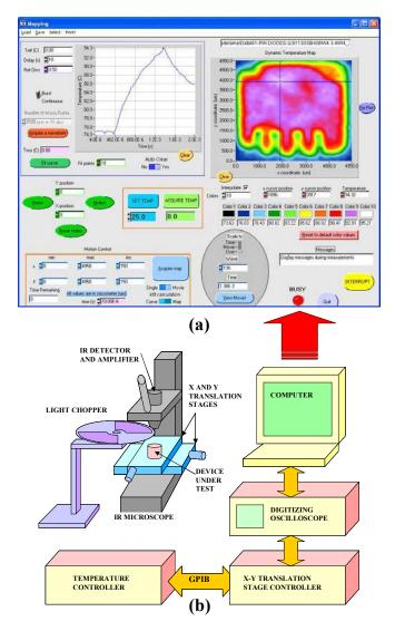
Figure 3. Transient Thermal Current Uniformity Degradation System: (a) front panel user interface, (b) experimental setup.
