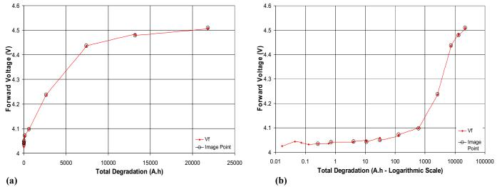
Figure 5. On-state voltage,  $V_f$ ; degradation as a function of total degradation (forward stress current-stress time product) for Diode 2: (a) regular scale, (b) logarithmic scale.
