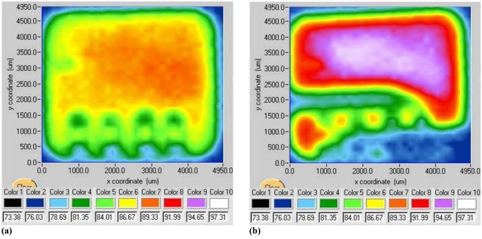
Figure 6. Thermal images for Diode 2: (a) first image before any degradation, (b) last image after 1000 degradation hours.
