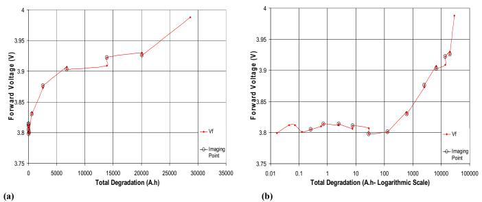
Figure 7. On-state voltage,  $V_{f}$ , degradation as a function of total degradation (forward stress current-stress time product) for Diode 4: (a) regular scale, (b) logarithmic scale.
