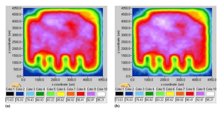
Figure 8. Thermal images for Diode 4: (a) first image before any degradation, (b) last image after 1000 degradation hours.
