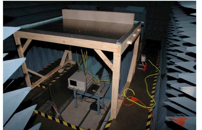
Fig. 5. Array configuration in anechoic chamber with concrete block wall on the border of the array and an absorbing border on the ground plane.
