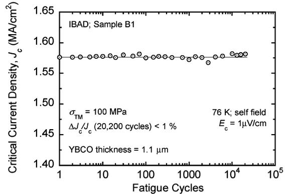
Fig. 3. Dependence of critical-current density  $J_c$  on fatigue cycling under transverse compressive stress up to 100 MPa and 20,200 cycles, in a non-Cu-plated YBCO IBAD slit coated-conductor. The fatigue effect is negligible, showing that propagation of edge cracks induced by conductor slitting is extremely limited.
