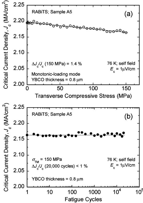
Fig. 1. Dependence of critical-current density  $J_c$  on (a) transverse compressive stress and (b) fatigue cycling up to 150 MPa and 20,000 cycles, in a neutral-axis YBCO RABiTS slit coated-conductor. Both effects are negligible, showing that transverse compression and fatigue cycling do not exacerbate edge cracks induced by conductor slitting.
