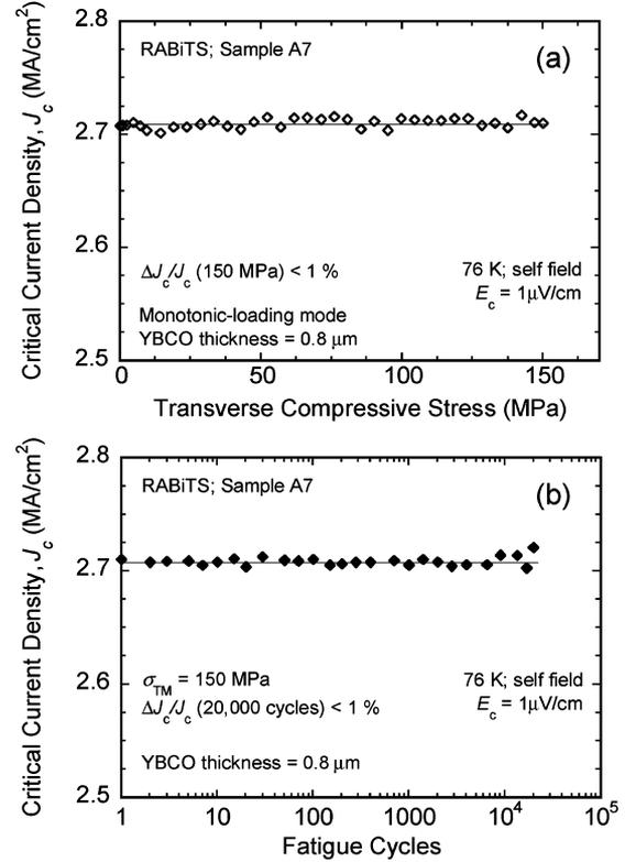
Fig. 2. Dependence of critical-current density  $J_c$  on (a) transverse compressive stress and (b) fatigue cycling up to 150 MPa and 20,000 cycles, in a 3-ply YBCO RABiTS slit coated-conductor. Both effects are negligible, again showing that transverse compression and fatigue cycling do not exacerbate edge cracks induced by conductor slitting.
