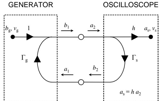
Fig. 1. Microwave flow diagram describing the propagation of signals between a generator and an oscilloscope. The generator on the left injects the signal  $b_g$  with no distortion, as indicated by the unity transfer function at the left of the flow diagram, into the circuit. The signal delivered to the oscilloscope is modified by the transfer function  $h$ , as well as being reflected multiple times by  $\Gamma_g$  and  $\Gamma_s$ .
