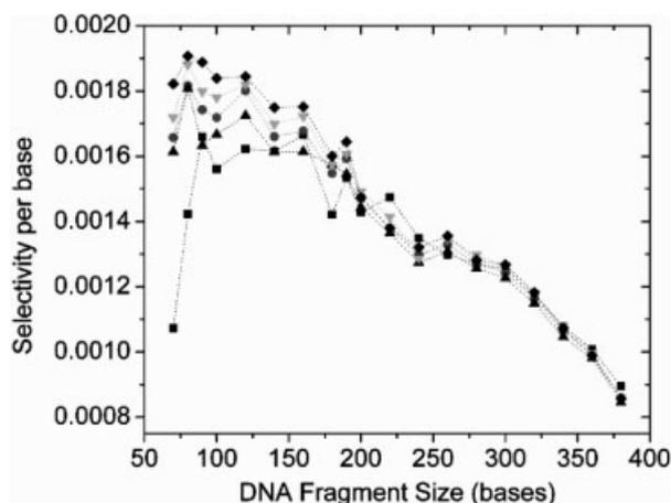
**Figure 6.** Selectivity of ssDNA fragments as a function of DNA fragment size, obtained for different surface treatment protocols. (■) 40DEA-60DMA coating, (▼) 15 min UV irradiation followed by HPMC coating, (▲) 10 min UV irradiation followed by HPMC coating, (●)  $\text{HNO}_3$  followed by HPMC coating, (◆) 10 min UV irradiation followed by PVA coating. The lines are drawn to guide the eye.
