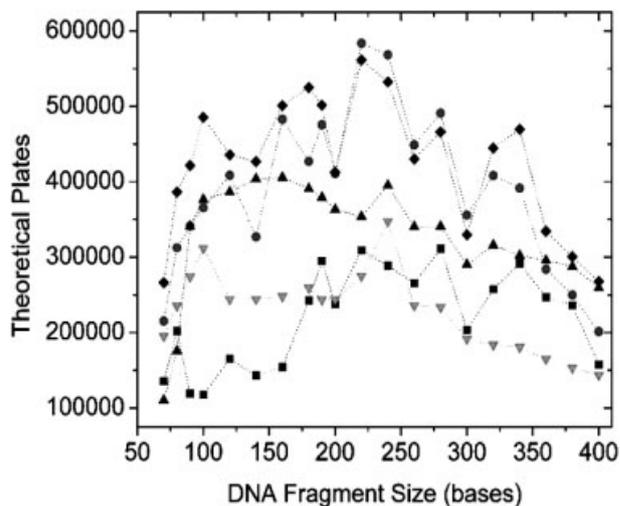
**Figure 5.** Theoretical plate count of ssDNA fragments, obtained for different surface treatments protocols. (■) 40DEA-60DMA coating, (▼) 15 min UV irradiation followed by HPMC coating, (▲) 10 min UV irradiation followed by HPMC coating, (●) HNO<sub>3</sub> followed by HPMC coating, (◆) 10 min UV irradiation followed by PVA coating. The lines are drawn to guide the eye.
