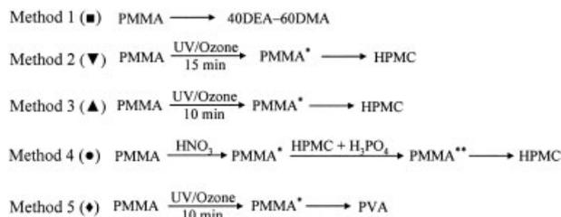
**Figure 2.** Schematic representation of the surface treatments investigated in the PMMA microchannel. Asterisks indicate modified surface.
