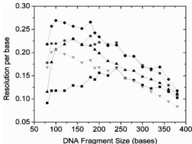
**Figure 7.** Resolution of ssDNA fragments as a function of DNA fragment size, obtained for different surface treatments and polymer coatings. (■) 40DEA-60DMA coating, (▼) 15 min UV irradiation followed by HPMC coating, (▲) 10 min UV irradiation followed by HPMC coating, (●)  $\text{HNO}_3$  followed by HPMC coating, (◆) 10 min UV irradiation followed by PVA coating. The lines are drawn to guide the eye.
