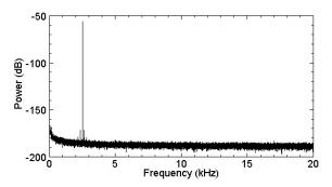
Figure 1. Digitally sampled spectral measurement showing -124 dBc [dB below the fundamental (carrier)] low distortion of the acJVS output. Just one Josephson array in the acJVS is generating a 50 mV (rms) sinewave at 2.5 kHz. The digitizer used 1 M $\Omega$  input impedance on the 10 V scale, 1 Hz resolution bandwidth, 10 averages, and a 100 KS/s sampling rate.
