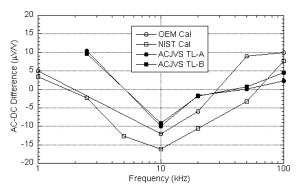
Figure 2. AC-DC differences vs. frequency for the same transfer standard. Solid symbols denote two acJVS measurements with the transfer standard floating (A) and grounded (B). Open symbols denote conventional calibrations.
