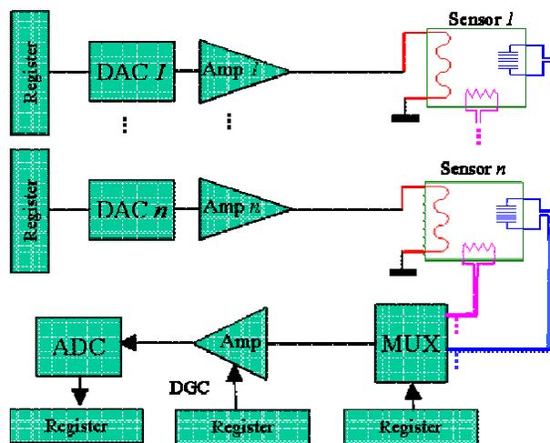
**Figure 2.** Gas-sensor Virtual Component (VC).
