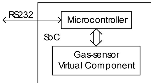
**Figure 1.** Gas-sensor SoC system architecture.
