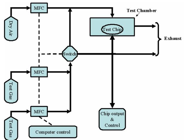
Figure 6. A schematic diagram of the gas handling capability used with the characterization system.
