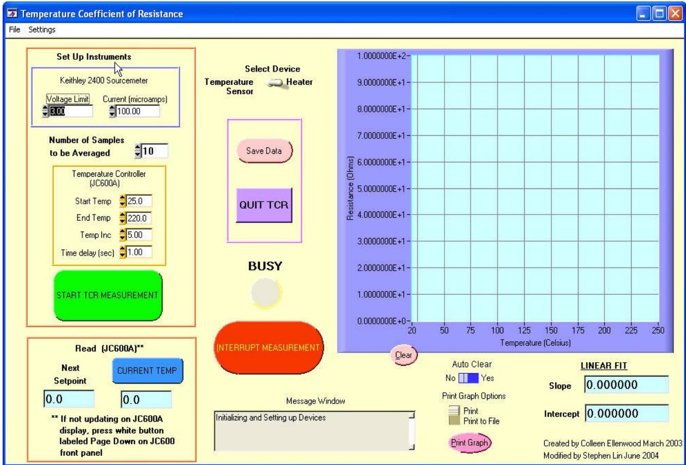
Figure 5. Virtual instrument user interface for microhotplate temperature-sensor and heater calibration
