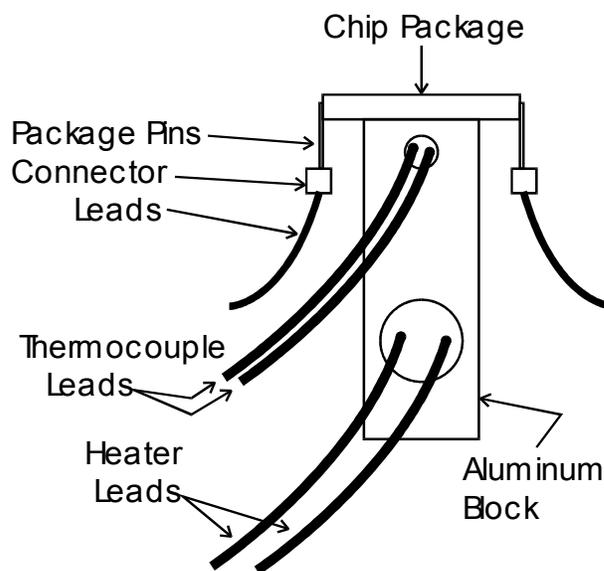
**Figure 4.** Microhotplate temperature-sensor calibration.
