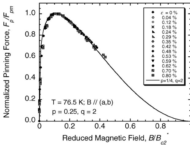
Fig. 6. Normalized pinning force density as a function of reduced magnetic field ( $b = B/B_{c2}^*$ ) at 76.5 K for a Cu-laminated YBCO coated conductor for various values of axial tensile strain up to 0.8%.  $B_{c2}^*$  is the effective upper critical field at which  $F_p(B)$  extrapolates to zero. Data show scaling of the pinning force density with reduced field for all the values of strain measured. The continuous line represents a function proportional to  $b^{0.25}(1-b)^2$ .
