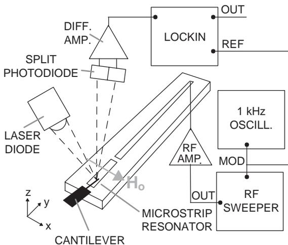
Fig. 1. A schematic of the experimental apparatus. The length of the cantilever is parallel to the resonator ( $y$ -direction). The bias field  $H_0$  is applied perpendicular to the resonator ( $x$ -direction).
