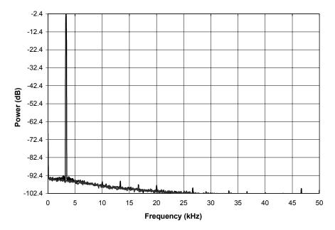
FIGURE 2. Spectrum analyzer measurement demonstrating -95 dBc low distortion for the ACJVS with two Josephson arrays generating a 242 mV (zero-to-peak) sinewave at 3.3 kHz using 8200 junctions at 10 Gbit/s. The spectrum measurement used 100 Hz resolution bandwidth and 100 averages.
