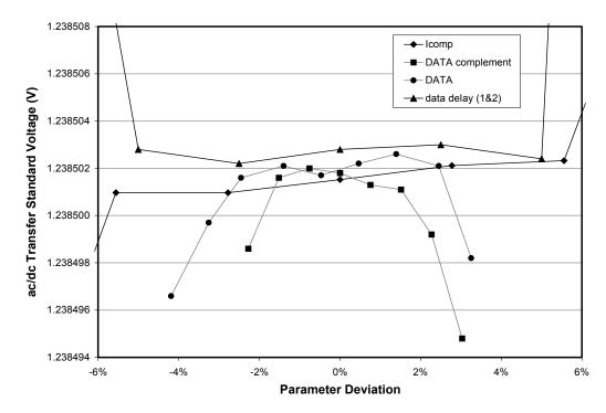
FIGURE 3. Plot showing the operating margins obtained at 8 Gbit/s using the ac/dc transfer standard and illustrating the "flat spots" for the 4 tightest parameters: amplitude (data), amplitude (data complement), data delay (both 1 & 2 moved together), and  $I_{comp}$ . One vertical division in this graph represents about 1.6 parts in 10<sup>6</sup>.
