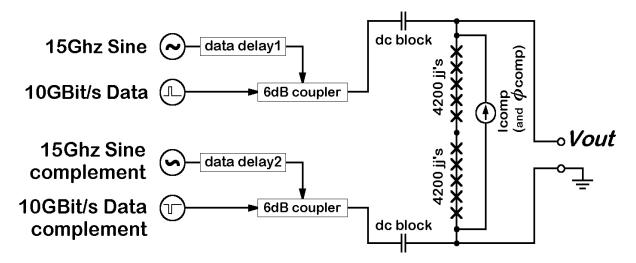
FIGURE (1) Diagram showing the system configuration and 8 individual bias parameters for the ACJVS system based on a chip containing two Josephson arrays.
