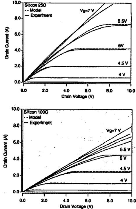
Fig. 8. Silicon MOSFET simulated (dashed) and measured (solid) output characteristics as a function of gate voltage for (a) 25 °C and (b) 100 °C.
