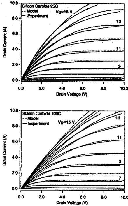
Fig. 7. Silicon carbide MOSFET simulated (dashed) and measured (solid) output characteristics as a function of gate voltage for (a) 25 °C and (b) 100 °C.
