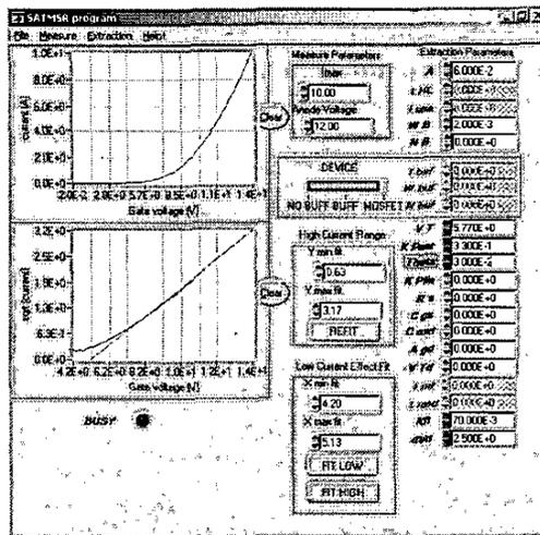
Fig. 3. SATMSR front panel demonstrating extraction of  $K_p$ ,  $V_T$ ,  $\theta$ ,  $K_{fl}$ , and  $dV_{Tl}$ .
