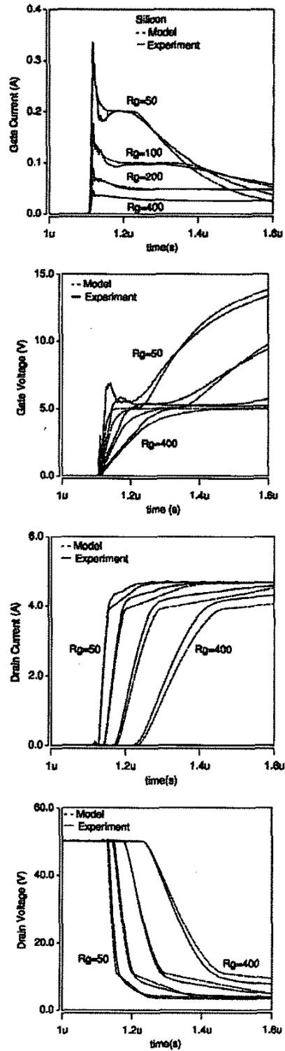
Fig. 10. Silicon MOSFET simulated (dashed) and measured (solid) turn-on waveforms as a function of gate resistance: (a) gate current, (b) gate voltage, (c) drain current, and (d) drain voltage.
