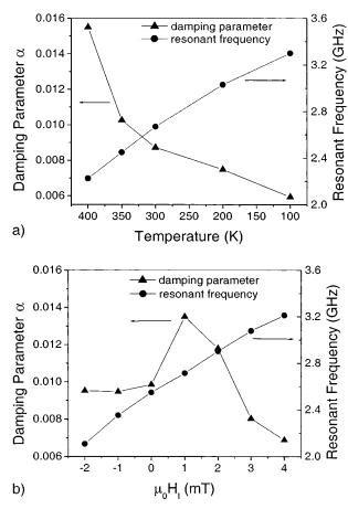
FIG. 4. The resonant frequencies and damping parameters determined from fitting the noise data for (a) the temperature-dependent data with no applied longitudinal field, and for (b) the longitudinal field dependent data at 300 K.
