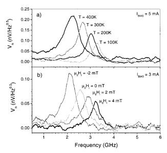
FIG. 1. Voltage noise spectra of a 1  $\mu$ m×3  $\mu$ m spin valve device for (a) a series of substrate temperatures with no applied longitudinal field, and (b) a series of longitudinal bias fields at room temperature. Both sets of curves are similar, with the resonant frequency increasing and the noise amplitude decreasing as the stiffness fields increase.
