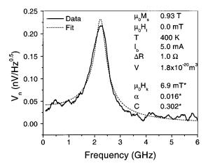
FIG. 2. Fit of the noise spectrum of a spin valve device at 400 K with a bias current of 5 mA. The parameters indicated with an asterisk were allowed to vary. The other parameters were taken from experimental measurements.
