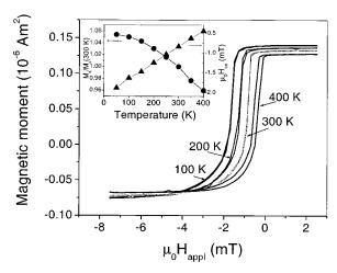
FIG. 3. Magnetic moment as a function of applied field for a coupon from the spin valve wafer. The field was applied parallel to the fixed-layer magnetization. The hysteresis loops are not centered around zero moment because of the fixed moment of the pinned layer. The inset shows the measured coupling field and relative free layer saturation magnetization calculated from the hysteresis loops.
