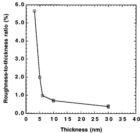
FIG. 2. Roughness-to-thickness ratio as a function of film thickness. Root-mean-square roughness values were used.
