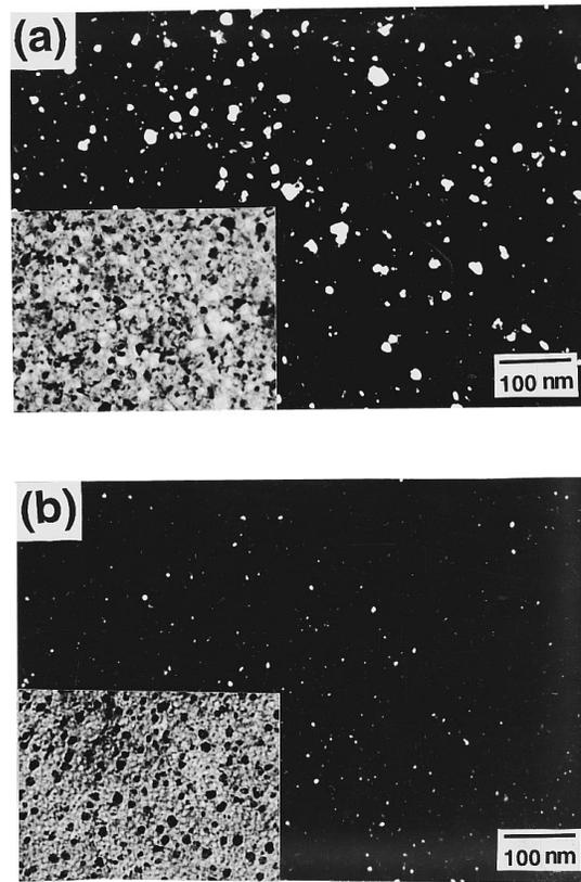
FIG. 3. TEM dark-field images depicting grain size and distribution (inset shows bright-field images) of (a) 30 nm film, and (b) 3 nm film.
