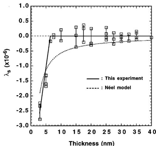
FIG. 1. Magnetostriction  $\lambda_s$  as a function of film thickness. The dashed curve is based on the Néel model.
