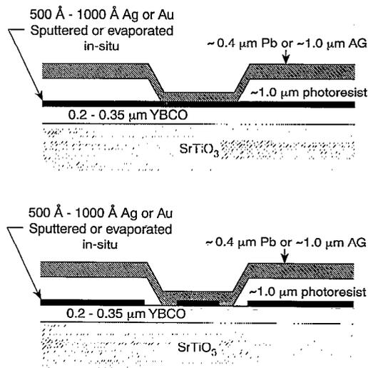
FIG. 1. Contact test geometries: (a) Window made in photoresist insulating layer with replaceable counter electrode of Pb or Ag. (b) Patterned *in situ* contact pad within photoresist window to eliminate spreading conductance into the surrounding *in situ* noble metal region (shown as black region in figure).
