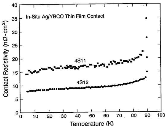
FIG. 3. Temperature dependence of specific contact resistivity  $\rho_c$ , showing only a 25% rise in  $\rho_c$  of high-quality *in situ* contacts from 4 to 90 K.
