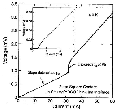
FIG. 2. Voltage vs current characteristic of  $2 \times 2 \mu\text{m}^2$  *in situ* Ag/YBCO contact showing 0.4 mA supercurrent (insert) and extensive ohmic region to more than 30 mA ( $> 10^6$  A/cm<sup>2</sup> transport current density through contact) before reaching the  $J_c$  of the Pb counterelectrode. Values of the specific contact resistivity  $\rho_c$  given in Table I were determined from this extensive linear region.
