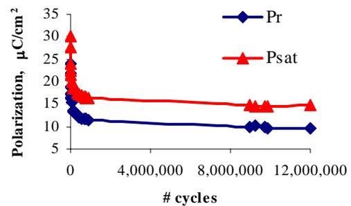
Figure 6. Change in polarization for a component processed at 1300 °C.
