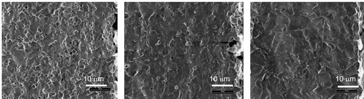
*Figure 3. SEM micrographs of fractured cross-sections for devices processed at 1175, 1250, and 1325 °C (from left to right), illustrating the evolution of the microstructure.*
