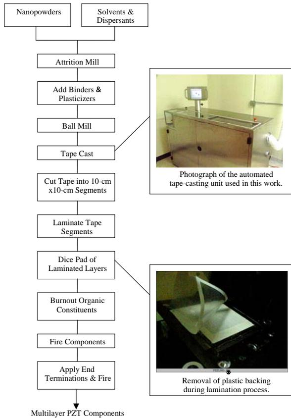
Figure 1. The actuator fabrication process.
