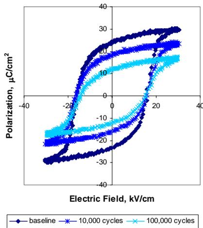
Figure 4. Change in P-E loops during the first 45 minutes of testing for a typical specimen processed at 1250 °C.
