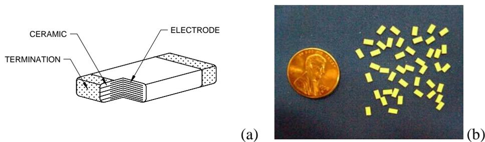
Figure 2. Schematic showing internal layers (a), and green parts diced from the pad (b).
