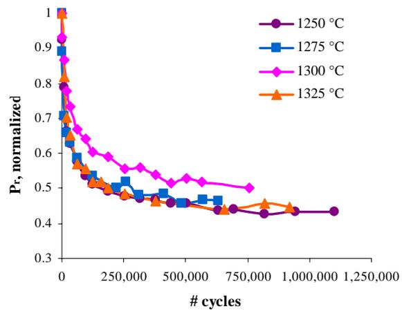
Figure 5. Degradation in  $P_r$  as a function of cumulative cycles for specimens processed from 1175 to 1250 °C (a) and 1250 to 1325 °C (b). Specimens sintered at 1175 °C were tested to only 500,000 cycles. Data shown are for a typical specimen at each temperature. Standard deviations ranged from  $\pm 0.38$  to  $\pm 6.06$  %.
