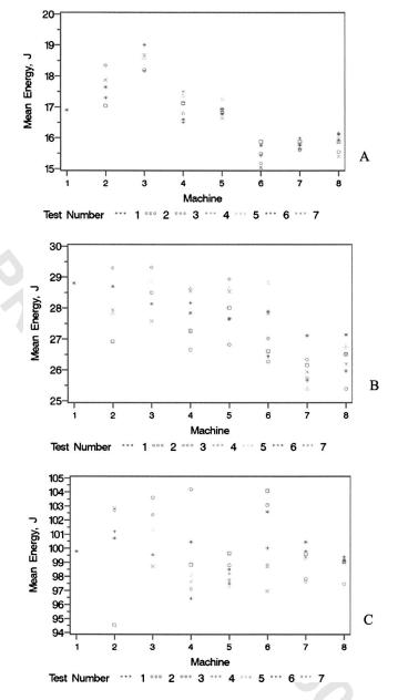
FIG. 3—The average energy of (a) low, (b) medium, and (c) high energy specimens is shown for each machine and test. Here the grouping of data for a given machine is most apparent. At low energy (a) the relative difference between machines and the lack of overlap for the data indicated clear differences due to the machines.
