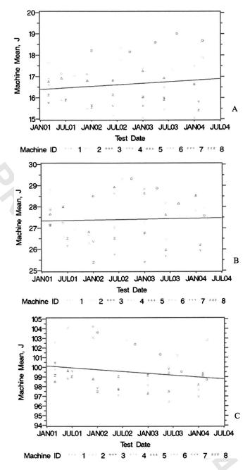
FIG. 1—The (A) low p=0.4, (B) medium p=0.8, and (C) high energy p=0.2 plots and probabilities showing trends for specimen stability.
