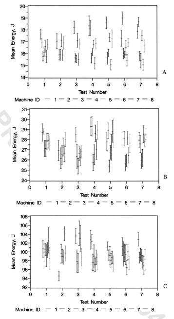
FIG. 2—*The average energy for each machine versus test number for: (A) low energy, (B) medium energy, and (C) high energy. Error bars are twice the standard deviation of the mean.*
