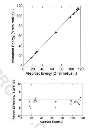
FIG. 4—A comparison of data for 8 and 2 mm striker geometries gathered by use of reference impact pendulums and type 4340 verification specimens. The upper plot (a) shows a general comparison, and the lower plot (b) shows the percent difference of the 8 and 2 mm striker data gathered on each machine (colors), for each set of verification specimens tested (the 2 mm data was subtracted from the 8 mm data, divided by the 8 mm data, and multiplied by 100).
