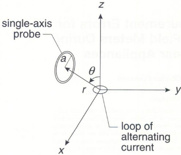
Fig. 1. A single-axis magnetic field probe with radius  $a$  is rotated until a maximum value of the dipole magnetic field produced by a small circular loop of alternating current is observed. It is assumed that the distance  $r$  is much greater than the dimensions of the loop.
