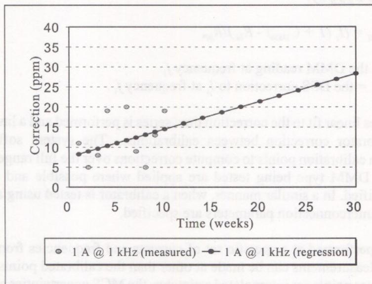
Fig. 11. Control chart with measured and predicted corrections for the MCS calibrator for ACI.
