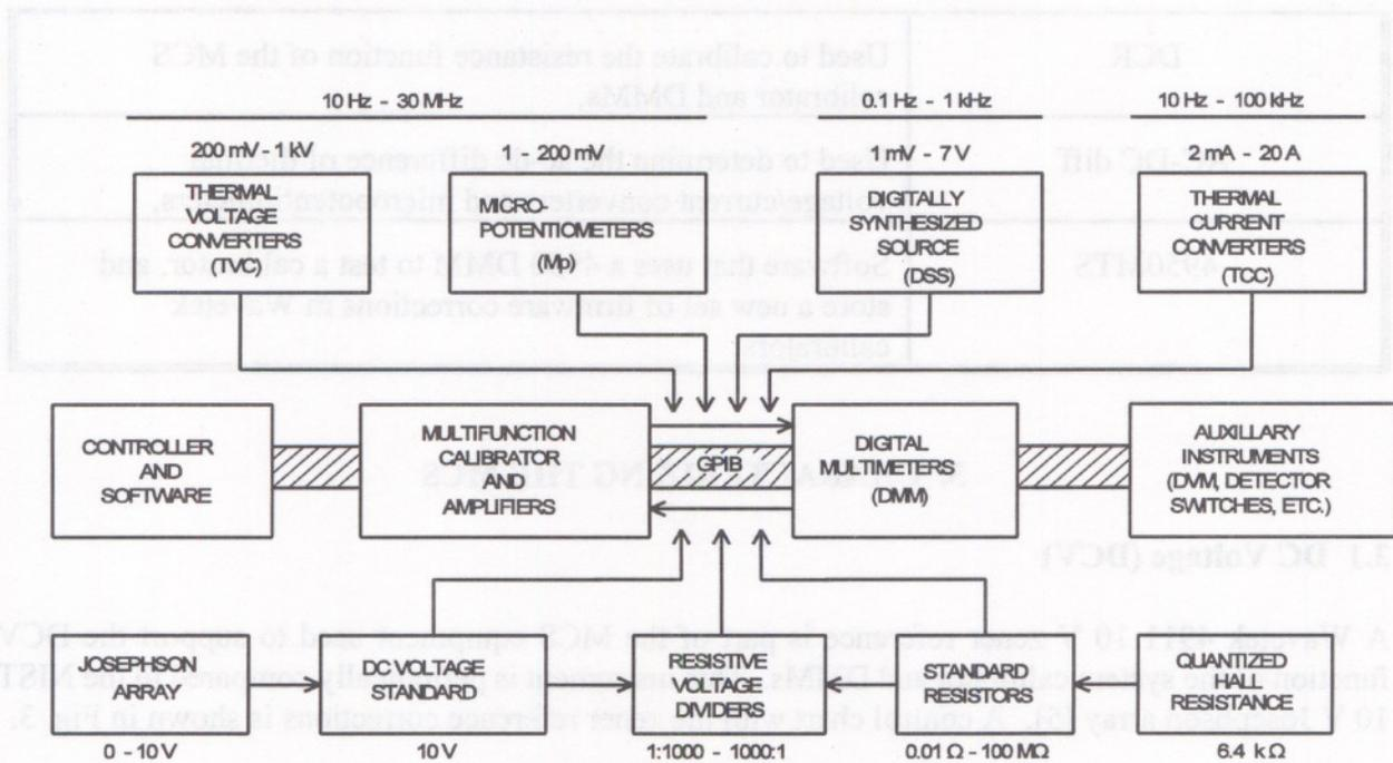
Fig. 2. Block diagram of MCS support equipment.
