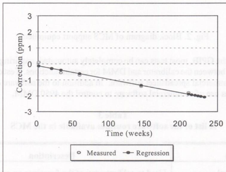
Fig. 3. Control chart with measured and predicted corrections for the zener reference.
