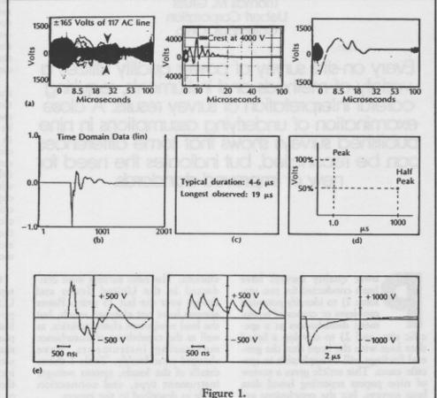
"Typical" waveforms reported in site surveys include three examples of surges recorded by Martzloff (a); typical waveform according to Goedbloed (b); description of waveform by Cannova (c); description of waveform by Odenberg-Braskich (d); and three examples of surges recorded by Wernstrom, Broms and Boberg (e)
