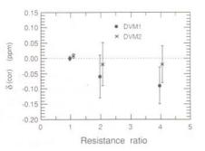
Fig. 3.  $\delta(cor) = \overline{d}_{DVM}(cor) - \overline{d}_{POT}$  results for 1:1, 2:1, and 4:1 resistance ratios using DVM1 and DVM2.  $\delta(cor)$  would be zero for exact agreement between the DVM and potentiometric methods. The data for DVM1 and DVM2 are slightly displaced for clarity.
