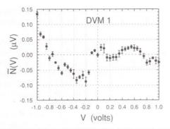
Fig. 2.  $\overline{N}(V)$  versus V curve for DVM1. The N(V) are the deviations in  $\mu V$  from the linear least-squares fit to the C(V) versus V data, as given by (7). The  $\overline{N}(V)$  are the averages obtained from six different Josephson array calibration runs.
