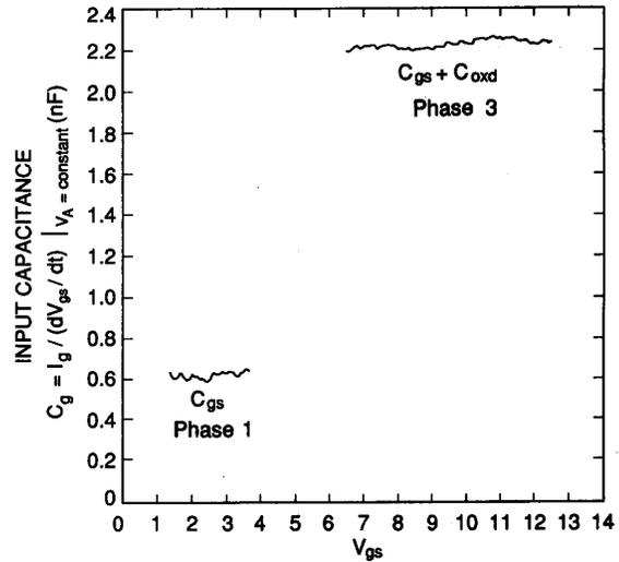
Fig. 7. Measured input capacitance versus gate voltage characteristics for  $V_{AA} = 300$  V obtained from digitized gate current and gate voltage waveforms similar to those in Fig. 6.
