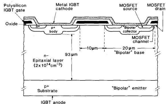
Fig. 1. Diagram of two diffused cells of n-channel IGBT.
