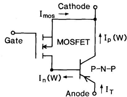
Fig. 2. Basic equivalent circuit model of IGBT.
