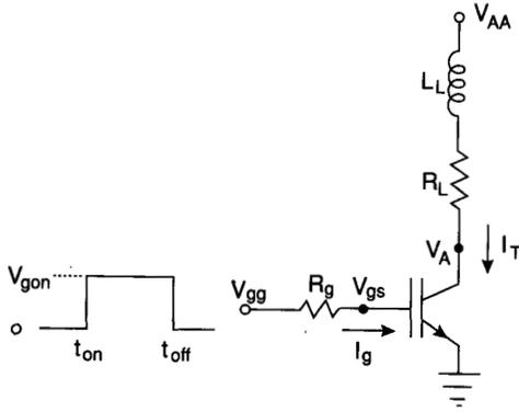
Fig. 5. Circuit configuration of IGBT with series resistor-inductor load and resistive gate drive.
