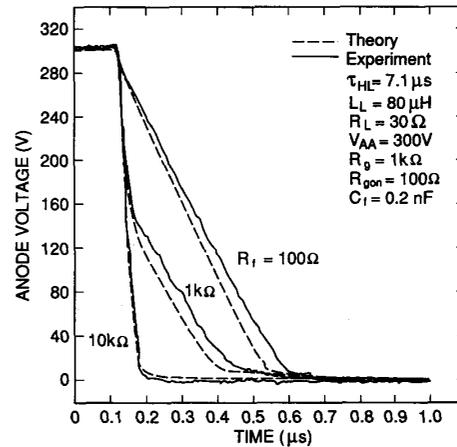
Fig. 14. Comparison of measured and simulated, anode voltage turn-on waveforms for circuit of Fig. 12 with different values of series feedback resistances.
