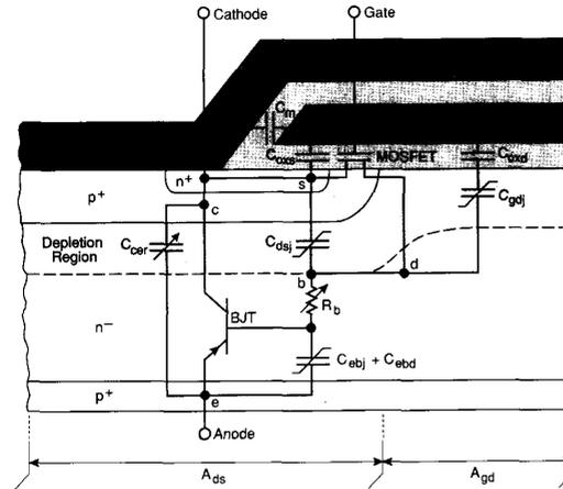
Fig. 3. Configuration of MOSFET and bipolar equivalent circuit components superimposed on schematic of one-half of symmetric IGBT cell.
