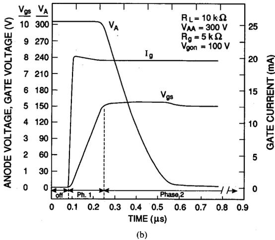
Fig. 6. Measured gate charging characteristics for low anode current and relatively constant ~20 mA gate current pulse where (a) is for  $V_{AA} = 20$  V and (b) is for  $V_{AA} = 300$  V.
