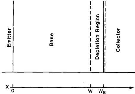
Fig. 4. Coordinate system used to develop IGBT bipolar transistor model. Emitter, base, and collector regions correspond to those indicated on right half of Fig. 1.
