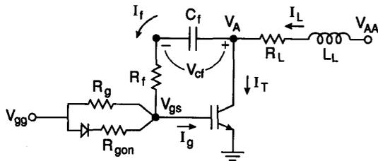
Fig. 12. Circuit configuration of IGBT with series resistor-inductor load, polarized gate drive resistance, and series resistor-capacitor feedback circuit.
