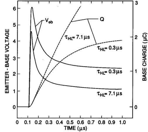
Fig. 11. Emitter-base voltage and base charge for same turn-on conditions as  $R_g = 10 \Omega$  waveform of Fig. 10 and for two different device base lifetimes.
