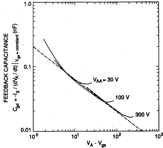
Fig. 8. Measured gate-drain feedback capacitance versus anode-gate voltage obtained from digitized gate current, gate voltage, and anode voltage waveforms similar to those in Fig. 6 for anode supply voltages of 30 V, 100 V, and 300 V.
