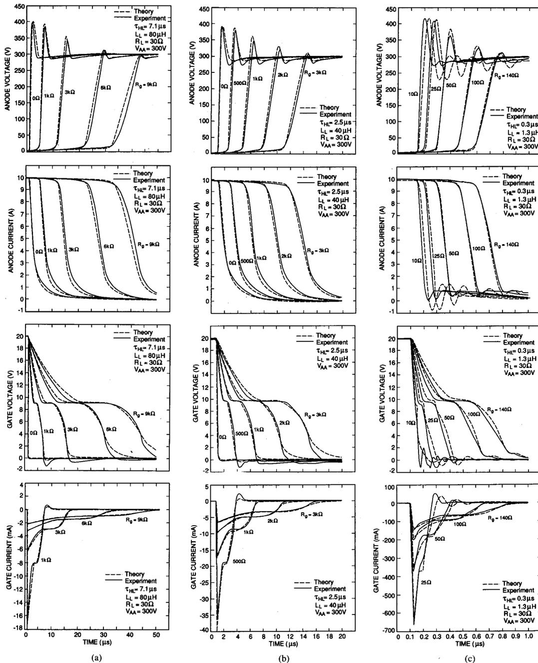
Fig. 9. Comparison of measured and simulated, gate and anode, current and voltage turn-off waveforms for the circuit of Fig. 5 with different values of gate resistance, where (a) is for 7.1- $\mu s$  device, (b) is for 2.5- $\mu s$  device, and (c) is for 0.3- $\mu s$  device.
