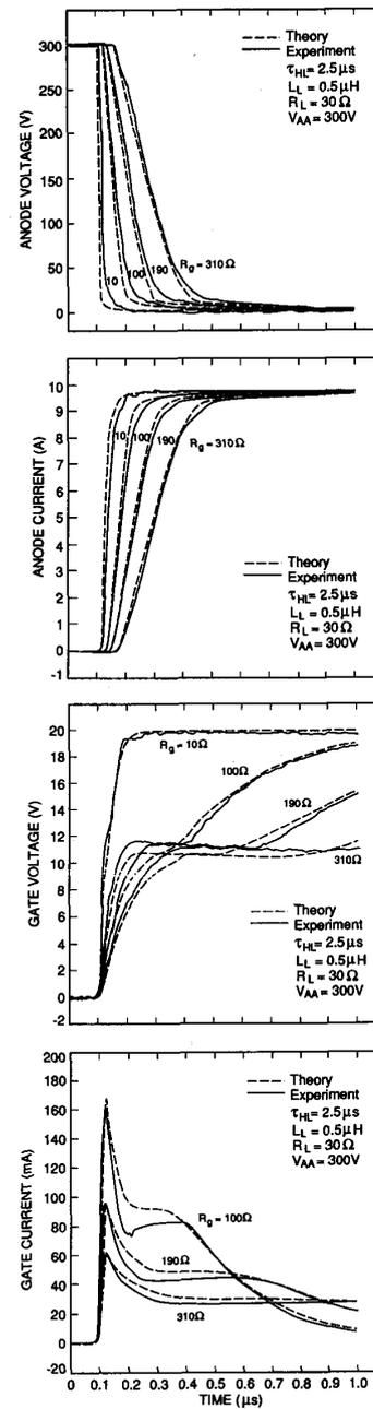
Fig. 10. Comparison of measured and simulated, gate and anode, current and voltage turn-on waveforms for circuit of Fig. 5 with different values of gate resistance.
