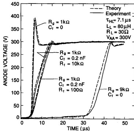
Fig. 13. Comparison of measured and simulated anode voltage turn-off waveforms for the circuit of Fig. 12 with different values of gate resistance, external gate-to-anode feedback capacitances, and different series feedback resistances.
