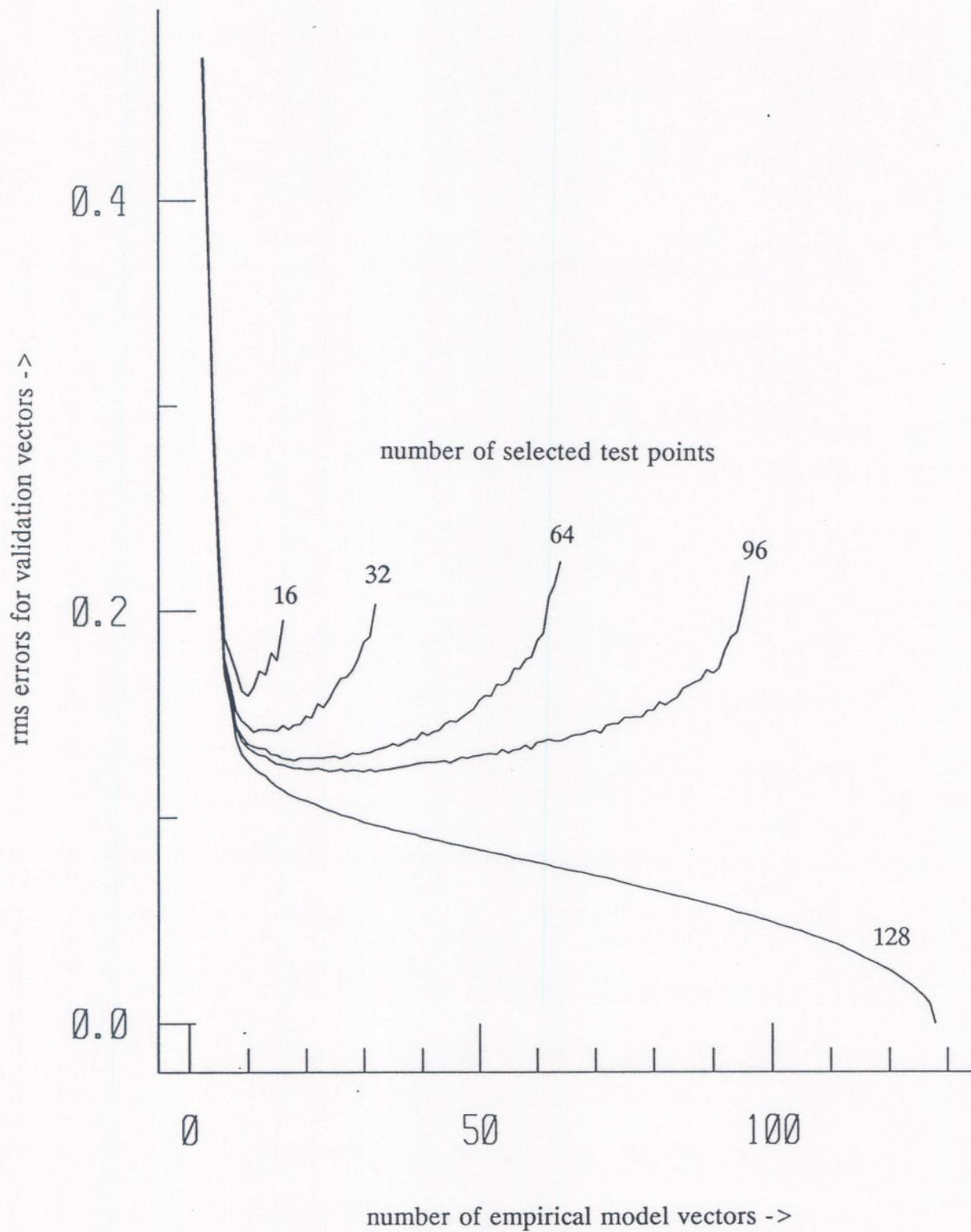
Figure 2. rms difference between predicted values and measured values using QRD derived models and an rms measurement noise of 0.1
