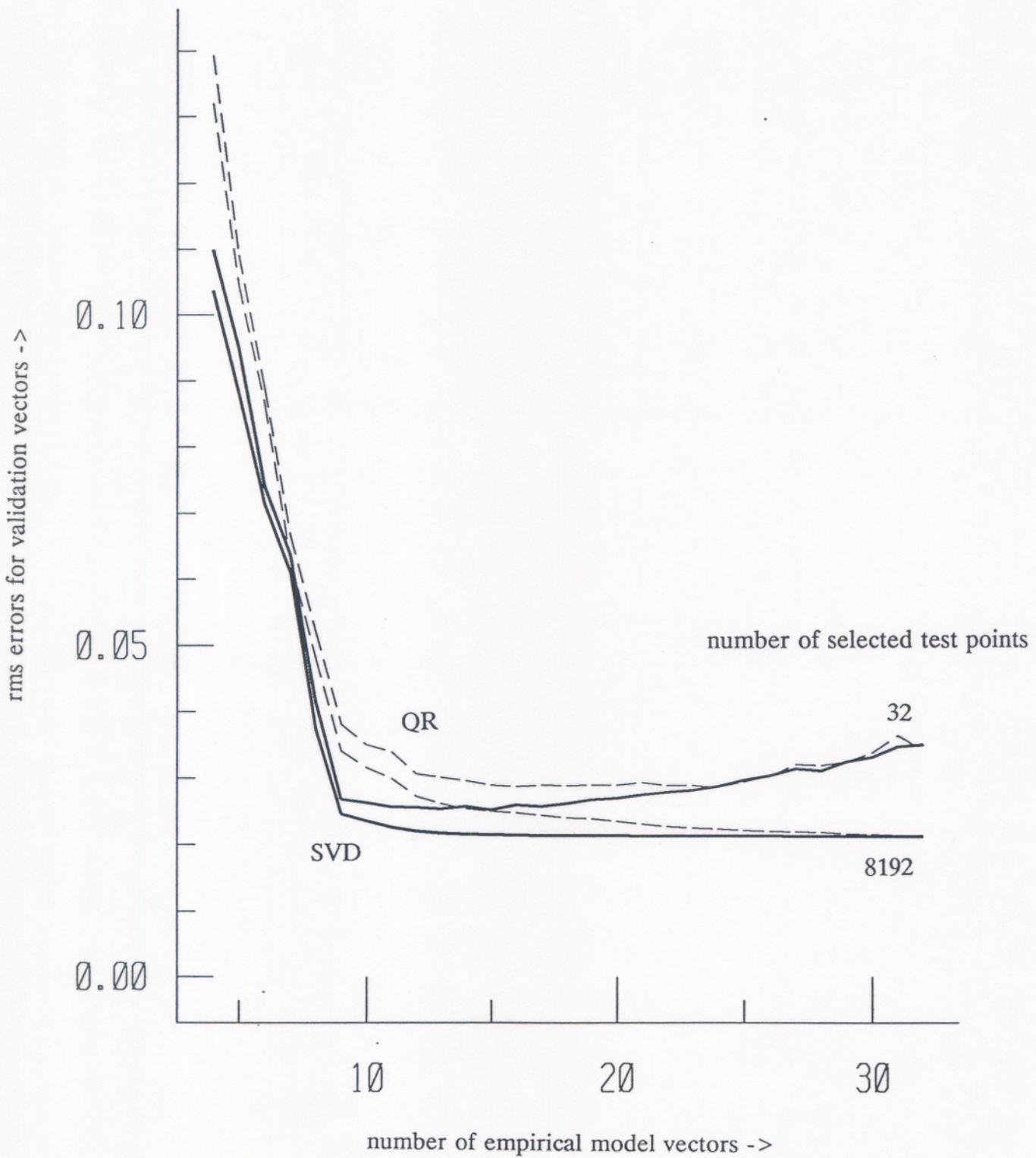
Figure 8. rms difference between predicted values and measured values using QRD and SVD derived models for data from a 13-bit A/D converter with an rms measurement noise of about 0.021
