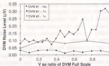
Fig. 3. A graph showing the noise levels in  $\mu$ V as calculated from the standard deviation of 10 DVM readings integrated over about 30 s. The x-axis is V as a ratio of full scale for various array voltages applied as input to the 1-V and 10-V ranges. Two different DVM models are represented. The noise level for both meters on the 0.1 V range is the same as that of DVM #1 on the 1-V range.
