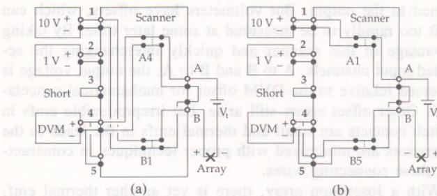
Fig. 2. A simplified internal wiring schematic illustrating two different switch configurations. (a) Selections A4 and B1. (b) Selections A1 and B5. To maintain the DVM polarity of the first circuit but interchange the array and 10-V source, the reverse DVM of channel 5 must be used.
