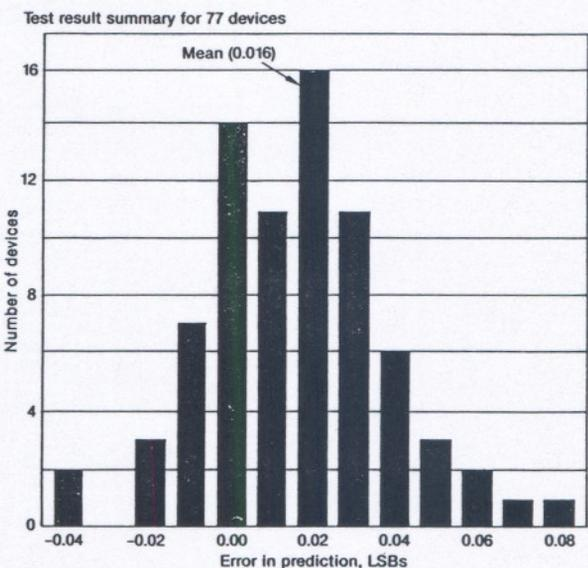
[5] The value of the new approach is best illustrated by this histogram, which illustrates the differences between the measured and predicted maximum integral nonlinearity for the 77 devices tested. For comparison, the standard deviation of the measurement process—the repeatability of each measurement—is 0.02 least-significant bit.
