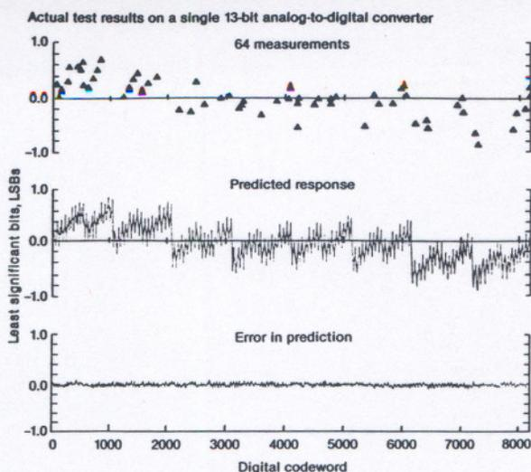
[4] Modeling works, as these results for a single analog-to-digital converter make clear. The top plot shows the integral nonlinearity measured at the 64 selected codes. The middle plot gives the predicted errors at all 8192 codes based on the 64 measurements, while the bottom plot gives the error in the predictions—the difference between the measured errors and the predicted errors at all codes. Vertical scales are in least-significant bits.
