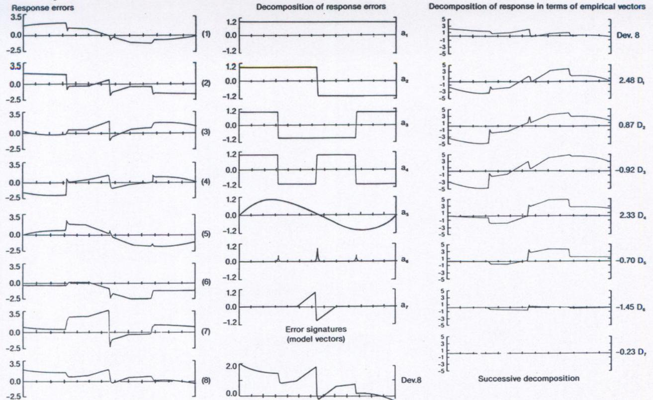
[1] The performance of a device as a function of one input condition can be illustrated by plotting the response error as a function of the input condition. In this case, the horizontal axis represents the digital output codes of a fictitious 7-bit analog-to-digital converter and the vertical axis is the input error corresponding to that code—the difference between the actual input that produced the digital code and the input that should ideally produce it. The scales are in arbitrary units.
