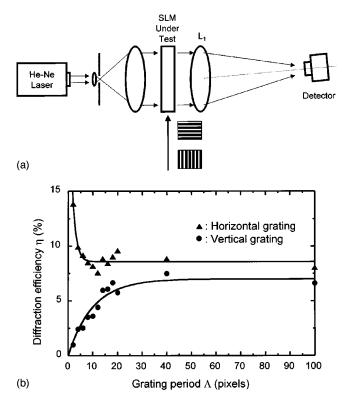
**Fig. 3** (a) Schematic diagram of an experimental setup to measure transfer function of SLMs and (b) transfer function of a type I SLM for horizontal gratings oriented along the fast scan direction (triangles) and vertical gratings along the slow scan direction (circles).
