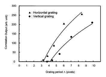
**Fig. 6** Correlation output versus grating period for input and reference patterns arranged along the vertical (triangles) and horizontal (circles) directions.
