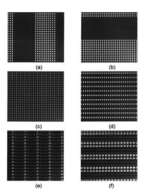
**Fig. 2** Experimental microscopic images of gratings with various orientations and periods: (a) to (d) were obtained with type I and type II LC SLMs and (e) and (f) were obtained with a type III LC SLM
