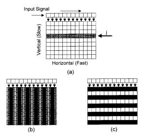
**Fig. 1** (a) Structure and addressing scheme of an electrically addressable SLM, (b) an SLM image of a vertical grating (the image is smeared along the fast scan direction), and (c) an SLM image of a horizontal grating (no smearing).
