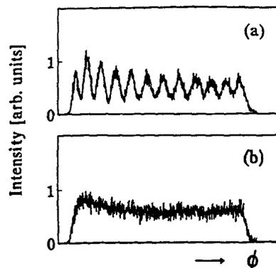
Figure 4: Polarization-sensitive detection of the scattered light (unnormalized): (a)  $\pi$ -polarized scattered light, showing interference, (b)  $\sigma$ -polarized scattered light, showing no interference (see text for explanation)
