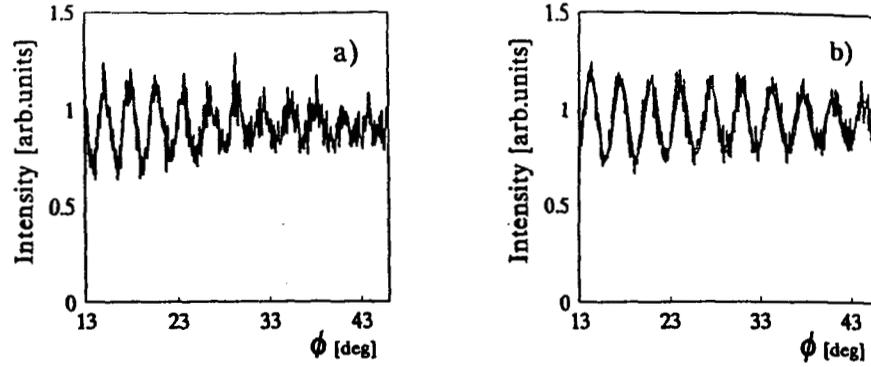
Figure 3: Shown are the interference fringes for a)  $d=3.9 \mu\text{m}$  and b)  $d=3.4 \mu\text{m}$ . Also shown in b) is a fit to the data (smooth line). From the fit we determined the temperature of the ions to be 1.5 times higher than the temperature at the Doppler cooling limit.
