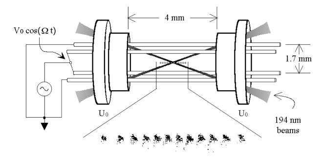
Figure 1: Linear rf trap, and an image of a string of twelve ions. The ions are spaced approximately  $10 \,\mu m$  apart. The spatial extent of the ions is exaggerated for clarity; in reality the laser beams overlap all of the ions.
