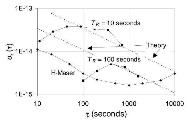
Figure 3: Stability plots for the 40.5 GHz microwave clock, using N = 13 ions, and both  $T_R = 10$  s and  $T_R = 100$  s. Also shown are the theoretically expected stabilities from Eq. (1), and the stability of the hydrogen maser reference clock.
