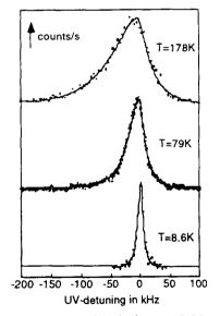
FIG. 2. Doppler-free two-photon spectra of the hydrogen 1S-2S transition observed in an atomic beam. The F = 1 hyperfine component has been recorded at different nozzle temperatures. The asymmetry and shift caused by second-order Doppler effects are greatly reduced at T = 8.6 K. (From reference [33].)
