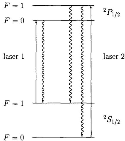
Figure 4. Energy level structure for the  $^2S_{1/2}$  and  $^2P_{1/2}$  levels of  $^{199}\text{Hg}^+$  near zero magnetic field. The  $^2S_{1/2}(F=0) - (F=1)$  hyperfine splitting is 40.5 GHz, and the  $^2P_{1/2}(F=0) - (F=1)$  hyperfine splitting is 6.9 GHz. The intervals are not drawn to scale. Lasers 1 and 2 are used for cooling, optical pumping, and detection as described in the text.
