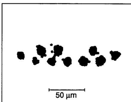
Figure 6. Image of a crystallized structure of ten  $^{199}\text{Hg}^+$  ions and one impurity ion. The potentials applied to the trap when this image was acquired were used as input for the numerical simulation shown in figure 3.
