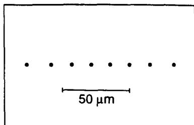
Figure 2. Numerical simulation of a crystallized string of eight  $^{199}\text{Hg}^+$  ions for secular frequencies  $\omega_r'/2\pi = 435$  kHz,  $\omega_z/2\pi = 41.7$  kHz. These secular frequencies were obtained by scaling secular frequencies measured under different conditions to the potentials applied to the trap when figure 5 was acquired.
