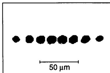
Figure 5. Image of crystallized string of eight  $^{199}\text{Hg}^+$  ions. The potentials applied to the trap when this image was acquired were used as input for the numerical simulation shown in figure 2.
