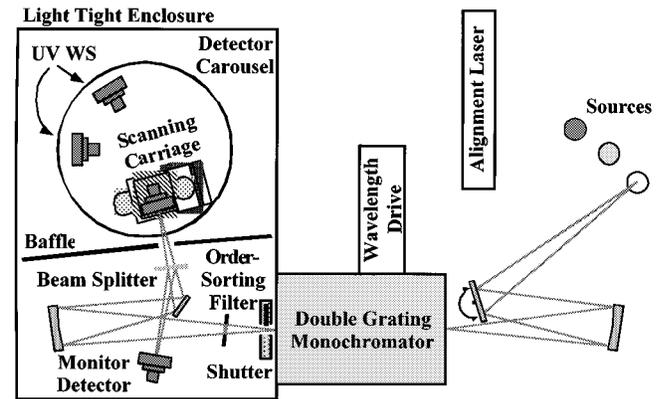
Fig. 1. UV SCF diagram. The irradiance meter-under-test is mounted on the scanning carriage. Spectral-responsivity comparison is accomplished by rotating the detector carousel to place one of the UV working standards (WS) into the beam. The order-sorting filter removes second-order light beyond 400 nm.
