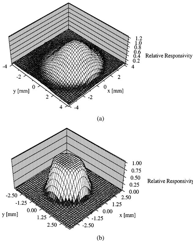
Fig. 3. Surface (3-D) plot of typical 365-nm detectors having different input geometries and diffuser materials. (a) Irradiance Meter #1. (b) Irradiance Meter #2.
