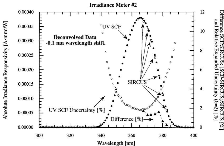
Fig. 5. Plot of irradiance responsivity, UV SCF relative expanded ( $k = 2$ ) uncertainties, and relative differences for the two methods for irradiance meter #2. Irradiance meter #2 is a NIST designed transfer standard with a  $\approx 25$ -nm bandpass (FWHM).
