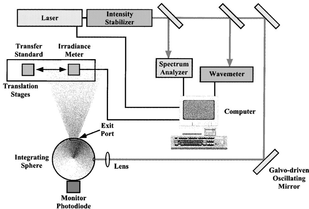
Fig. 2. SIRCUS diagram. The irradiance meter calibration is performed by direct substitution with the irradiance transfer standard.
