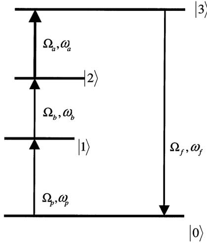
Fig. 1. Lifetime-broadened four-level atomic system interacting with two cw fields ( $\Omega_{a,b}; \omega_{a,b}$ ), and a weak pulsed pump field ( $\Omega_p; \omega_p$ ) to generate a FWM field ( $\Omega_f; \omega_f$ ).
