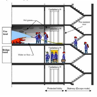
Figure 4 - firefighter lifts carry people and equipment to the floor below the fire with attack staged from the stairs<sup>9</sup>
