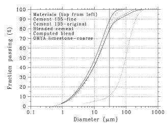
Fig. 1. Measured particle size distributions for materials used in this study.
