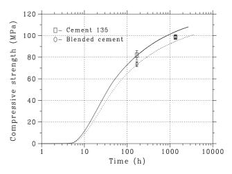
Fig. 4. Measured ( $\Box$  and  $\bigcirc$ ) and model (lines) compressive strength development for original cement (solid line) and blended system (dashed line) mortars with w/s=0.3 cured under saturated conditions at 25 °C. Error bars indicate plus or minus one standard deviation in the experimentally measured values.
