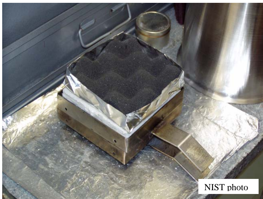
Figure D-2. Sample of Polyurethane Foam Placed in Aluminum Foil Tray on Top of Horizontal Sample Holder.
