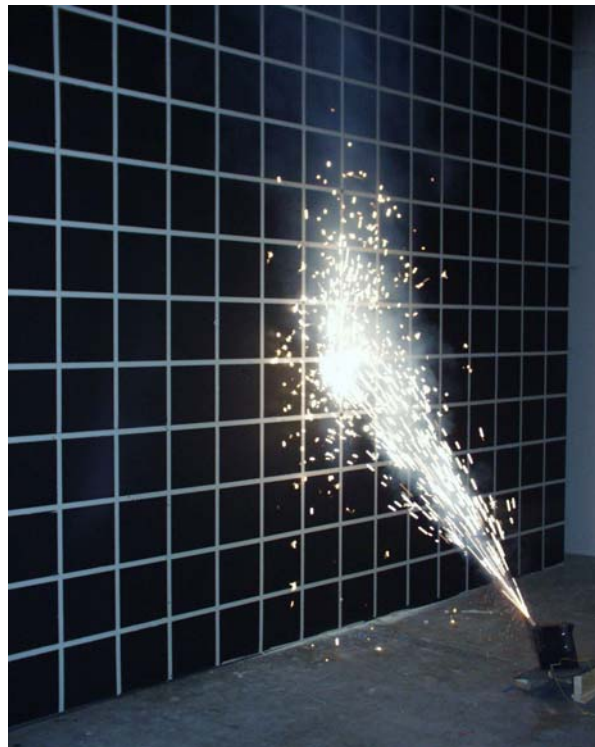
Figure F-4. Single Gerb at 45 degrees and in a Plane Perpendicular to Wall.
