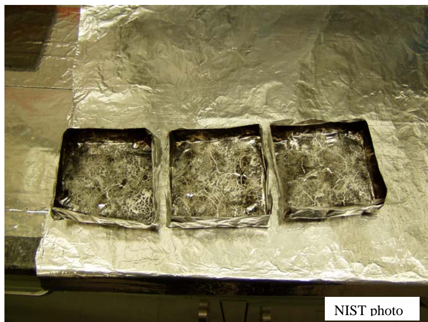
Figure D-4. Burn Residue of Polyurethane Foam after Cone Calorimeter Test.
