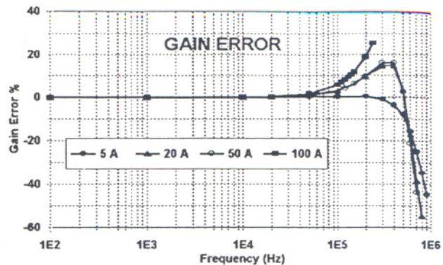
Fig. 5. Plot of gain error vs frequency for four ranges.
