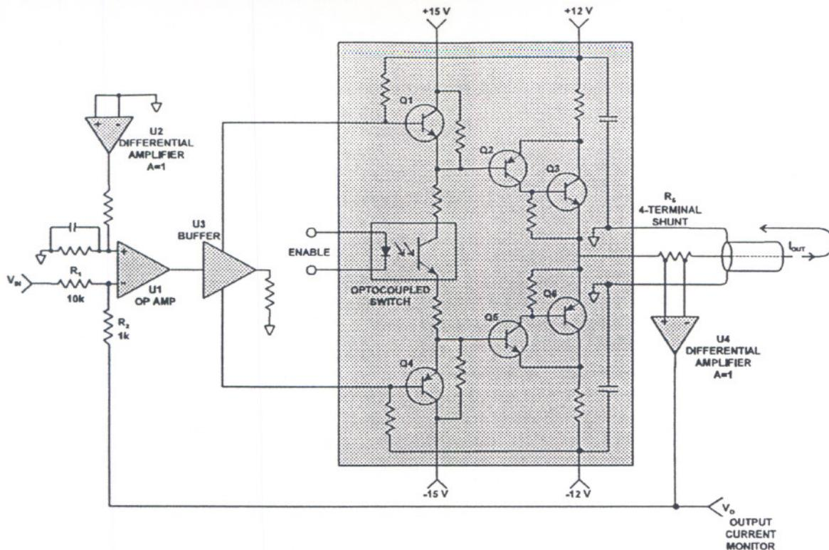
Fig. 2. Simplified schematic diagram of the 5 A transconductance amplifier.
