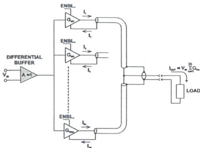
Fig. 1. Block diagram of the high current transconductance amplifier utilizing a parallel array of lower current transconductance amplifiers.
