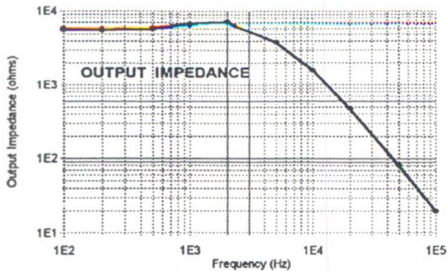
Fig. 4. Plot of output impedance vs frequency on the 5 A range.
