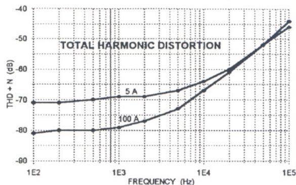
Fig. 3. Plot of total harmonic distortion plus noise vs frequency.
