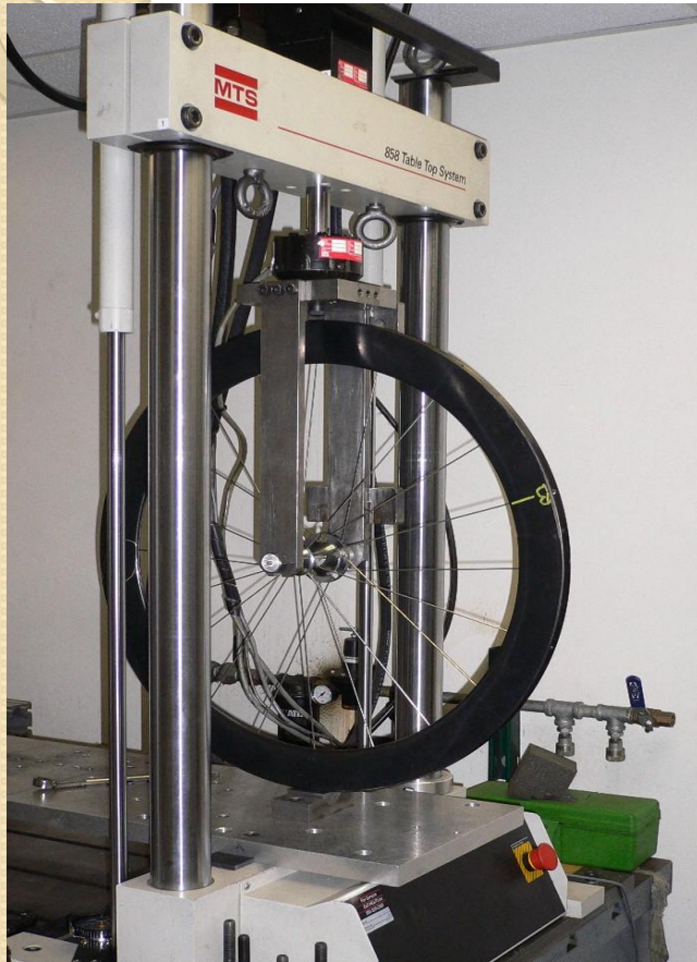
Composite wheel static and fatigue testing
