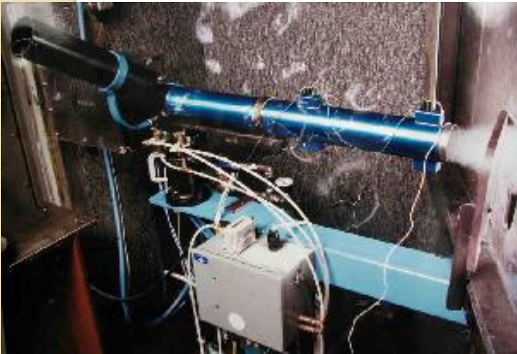
Bat Cannon –Repetitive impact at 110, 120, 130 mph
