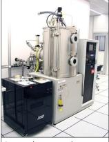
A second vacuum e-beam evaporator has been installed in the NanoFab cleanroom.
